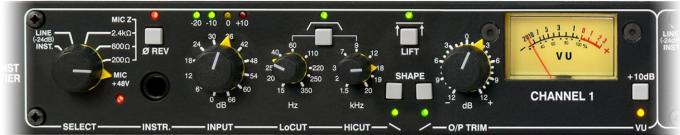
**SELECT** Instr./Line/Mic 2.4k,600 & 200 Ohm/Mic +48V The source select is a six position rotary switch that, as well as setting the input source, also sets the load impedance of the microphone.
